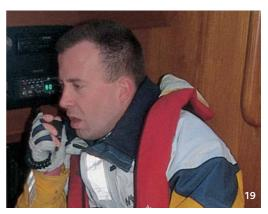
Do not rely solely on the DSC alert. It should be immediately followed by emergency radio procedures on VHF Channel 16.
